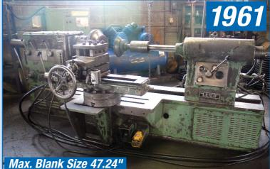
**LEIFELD** Model PLB 600, Max. Blank Size 47.24", Max. Blank Size in Gap 63", Width of Gap 19.7", Distance Between Centers 35.43", X Axis Travel 11.5", Z Axis Travel 25", Main Spindle Drive 15HP, Hydraulic Pump Motor 10 HP, Slide Power Longitudinal (Z) 9,920 lbf, Slide Power Transverse (X) 5,511 lbf, Spindle DIN 11, Tailstock Stroke 29.5", Mechanical and Hydraulic Top Slide, Ejector, sn 4954/XIII/3
