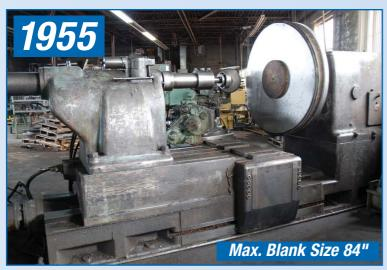
**BOKO** Model PIIIb-K 361/1, Max. Blank Size 84", Distance Between Centers 82.6", X Axis Travel 11.8", Z Axis Travel 39.3", Main Spindle Drive Upgraded to 40 HP, Upgraded Hydraulic Pump Motors Total 25 HP, Slide Power Transverse (X) 14,100 lbf, Tailstock Stroke 29.5", S.N. 275
