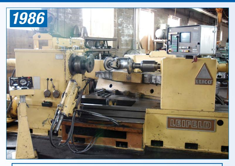
**LEIFELD** PNC 600, Max. Blank Size 47.24", Distance Between Centers 55.12", X Axis Travel – 19.69", Z Axis Travel – 27.56", Main Spindle Drive 40/30 HP, Hydraulic Pump Motor 33.5 HP, Slide Power Transverse (X) & Longitudinal (Z) 22,480 lbf (pound force), Tailstock Stroke 25.59", Ejector Stroke 15.75", Spindle Mount (Tool Adaptor) DIN 11, Including The Following Options: KA Unit, Material Support Device, Centering Unit, Roll Block System – Slide Lifting, 600V, Series 3/1, sn 10.1957.0
