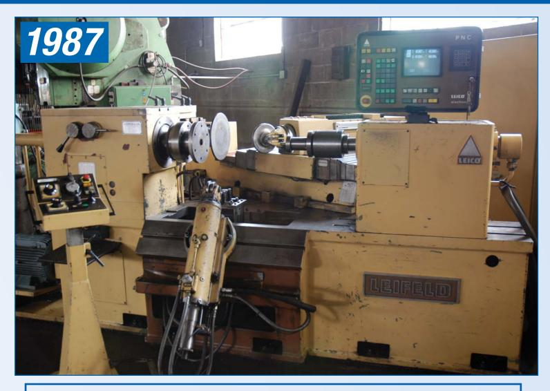
**LEIFELD** PNC 450, Max. Blank Size 35.43", Distance Between Centers 40.35", X Axis Travel – 12.20", Z Axis Travel – 19.69", Main Spindle Drive 25/15 HP, Hydraulic Pump Motor 28.5 HP, Slide Power Transverse (X) & Longitudinal (Z) 14,612 lbf, Tailstock Stroke 19.69", Ejector Stroke 11.81", Spindle Mount (Tool Adaptor) DIN 8, Including The Following Options: KA Unit, Material Support Device, Centering Unit, 600V, Series 20/1, sn 10.2224.0
