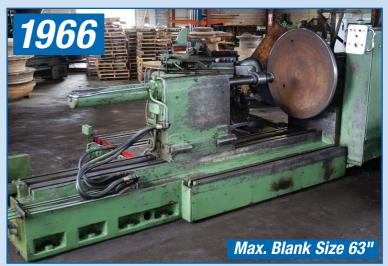
**BOKO** Model D82H, Max. Blank Size 63", Centre Height 32.3", Distance Between Centers 106", X Axis Travel 11.8", Z Axis Travel 49.3", Main Spindle Drive 40 HP, Hydraulic Pump Motor 7.5 HP + 1 HP, Slide Power Longitudinal (Z) 26,400 lbf, Slide Power Transverse (X) 20,000 lbf, Tailstock Stroke 35.4", 550V, sn 417
