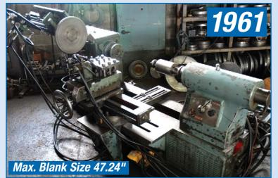
**LEIFELD** Model PLB 600, Max. Blank Size 47.24", Max. Blank Size in Gap 63", Width of Gap 19.7", Distance Between Centers 35.43", X Axis Travel 11.5", Z Axis Travel 25", Main Spindle Drive 15 HP, Hydraulic Pump Motor 10 HP, Slide Power Longitudinal (Z) 9,920 lbf, Slide Power Transverse (X) 5,511 lbf, Threaded Spindle M 89, DIN 800 – 3.5", Tailstock Stroke 29.5", Mechanical and Hydraulic Top Slide, Material Support Cylinder
